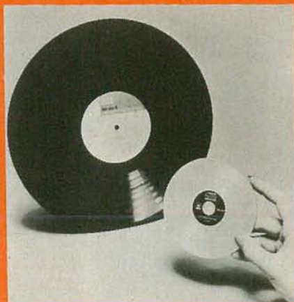
FIG. 1—THE 4.7-INCH DIAMETER C-DAD disc contains one hour of music on a side compared to a little over 20 minutes for a conventional 12-inch LP.
