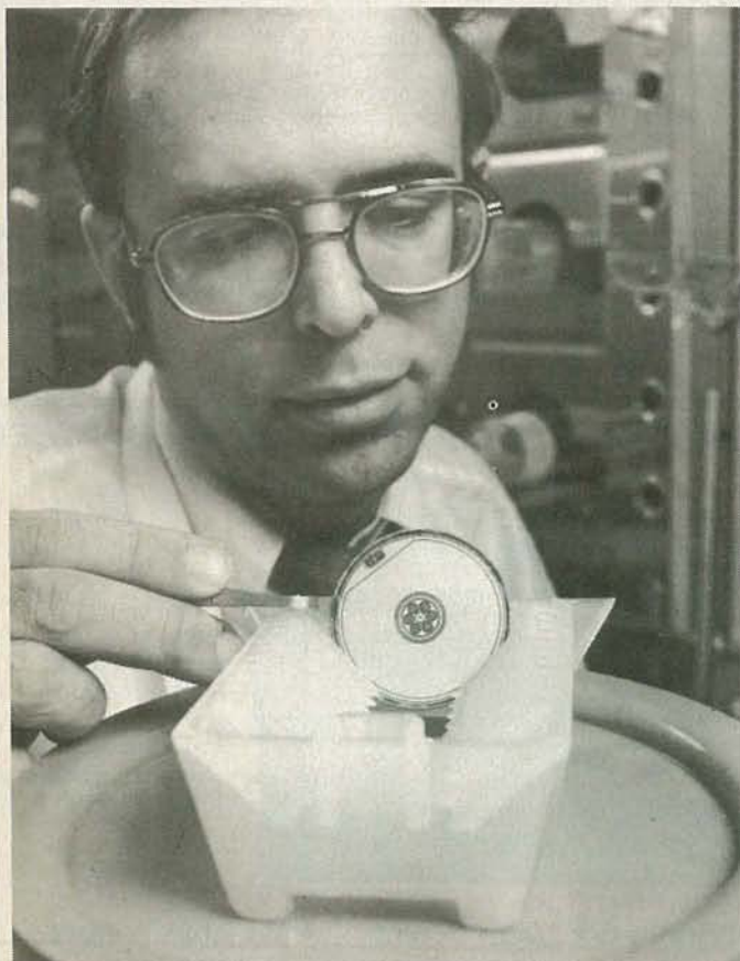
GE's NEW THYRISTOR, inspected here by Dr. Victor A.K. Temple, promises great reductions in high-voltage DC power-line costs. Through its innovative design, it can handle large currents while consuming little power itself, reducing the conversion losses of HVDC transmission systems. Work on the device, still in the early developmental stage, is being sponsored by the Electrical Power Research Institute, the research arm of the electric utility industry.
