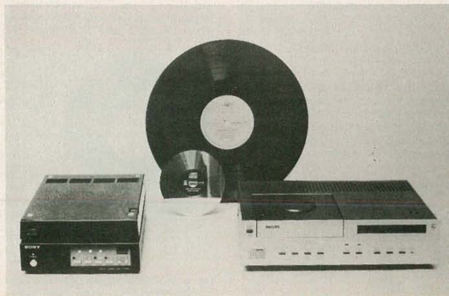
FIG. 3—C-DAD PLAYER prototypes shown in 1981. Sony's is at left; Philips' at right.
