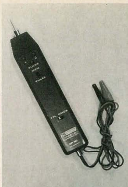
FIG. 3—SWITCH-SELECTABLE threshold levels (TTL/CMOS) are common on logic probes such as B&K-Precision's DP-50.
