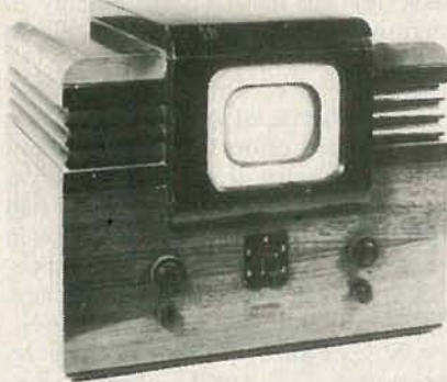
FIG. 4—THIS EARLY TELEVISION SET, the RCA model TT-5 , was one of the first offered for sale to the general public. It featured a five-inch screen, five-channel coverage, but no audio section; it sold for $199.50 in 1939.
